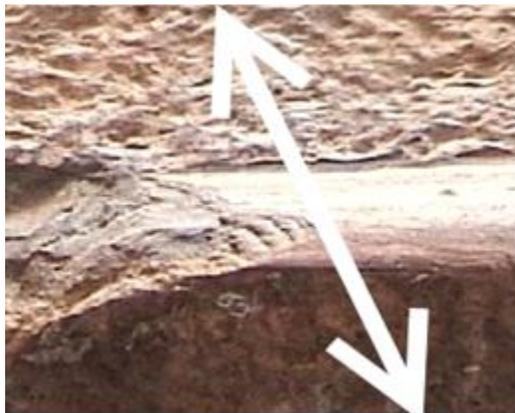
The white line indicates where the thin section was made. The smooth layer on the picture is about 2 cm wide and 1.3 cm deep. The sample was carefully cut into two parts and a thin section was taken for analysis in the Microprobe, jxa 8600 Pioneer. Several points were measured on the inside of the sample and on the smooth surface.
